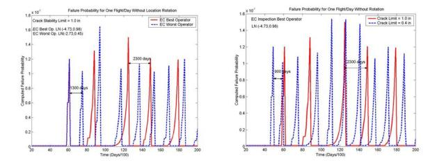
Figure 9. Risk-based Inspection Times for One-Flight/Day, Without Rotation and Given Target Risk of  $2x10^{-7}$ : a) Effect of the Operator's Skill and b) Effect of Crack Limit Criterion.
