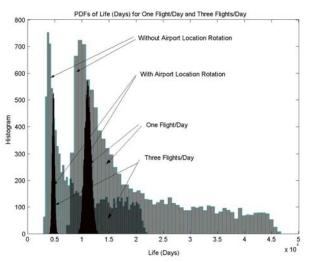
Figure 7. Corrosion-Fatigue Statistical Histograms for the Four Scenarios
