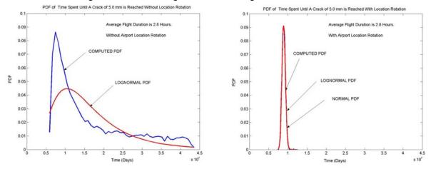
Figure 8. PDF of Corrosion-Fatigue Life for One-Flight/Day Without and With Airport Rotation
