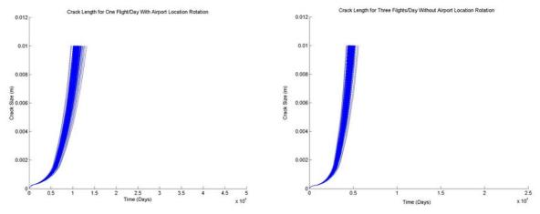
Figure 6. Simulated Crack Size Curves With Airport Rotation
