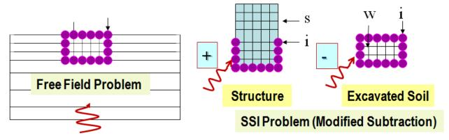
Figure 3. Modified Subtraction Method (MSM) Implementation (FI-EVBN in ACS SASSI)
