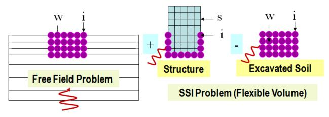
Figure 1. Flexible Volume or Direct Method (DM) Implementation (FV in ACS SASSI)
