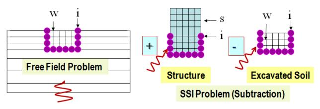
Figure 2. Subtraction Method (SM) Implementation (FI-FSIN in ACS SASSI)
