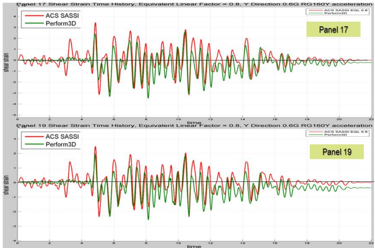
Figure 11 Story Drifts for Panels 17 and 19 Computed Using ACS SASSI Iterative Approach and PERFORM3D Time-Domain Integration Approach
